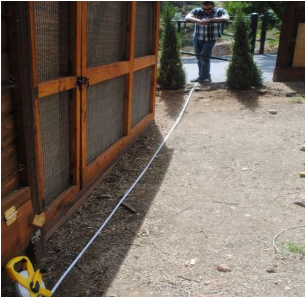
Interior road to structure corner (fencing does not constitute a structure).
