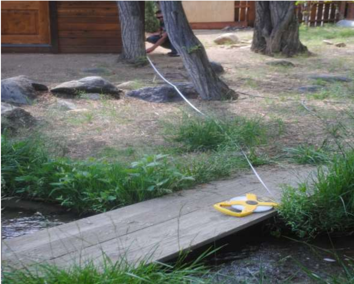
Northern corner measurement of structure corner to the irrigation ditch.
