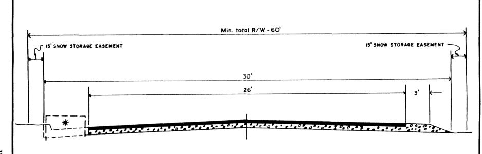
FIGURE 27 JUNE LAKE TYPICAL SECTION COLLECTOR/RESIDENTIAL
