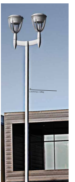
14' Pole with Acorn Fixture, similar to existing luminaires, for use along Main Street, 50' o.c. typ. 16.5' Pole with double Acorn fixture for use along Main Street, 100' o.c. typ. 20' Pole with drop acorn fixture for use along entry routes into Bridgeport, 100' - 200' o.c. typ.
